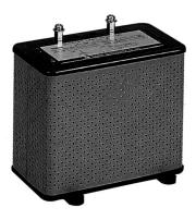
Current limit resistor(CLR) will make the grounding relay and zero voltage meter operate due to the current which in a djusted primary neutral side current when fault. And it will be connected with 3ry side of GPT between terminal "a" and terminal "f" and then it restrains the 3ry harm once voltage and abnormal potential.
